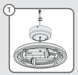
Feed the wires through the center hole in the switch housing, the washer, and the nut. Then install the switch housing by twisting clockwise onto the threaded rod. Install the washer and nut onto threaded rod and tighten securely.
